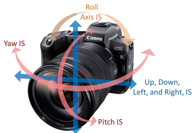
Figure 39 Showing the five dimensions of image stabilization correction in the EOS R camera
